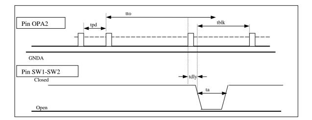
Timing for JMP2 =Vdd, Conditions for JMP2=open are similar
