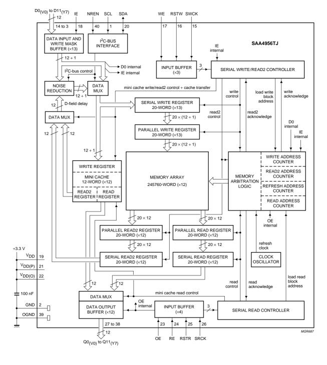
Pin 21 ( $V_{DD(P)}$ ) should be connected to the supply voltage of the driving circuit that generates the input voltages. This could be, for instance, 5.0 V instead of 3.3 V. Pins 19 and 22 ( $V_{DD}$  and  $V_{DD(O)}$ ) require a 3.3 V supply.
