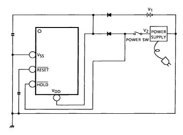
Note 10:  $V_1 = +3 \text{ V}$ : Battery supply
