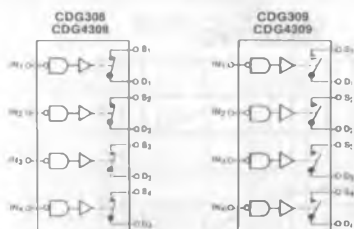
Four SPST Switches per Package Switches Shown in Logic "1" Input Position
