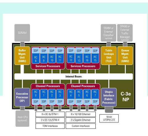
Highly-integrated NPU architecture provides programming efficiencies for advanced services in access applications
