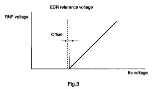
The pins are the inputs to a differential amplifier. A reference voltage of 1.0V (recommended value for BA6860FS) or 1.2V (recommended value for BA6862FS) is applied to pin 7. The offset voltage range is between -100mV and +100mV for the BA6860FS and between -150mV and +150mV for the BA6862FS. (3) Brake
